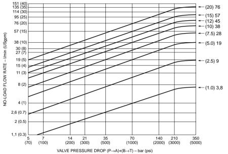
SPOOL RATED FLOW - (USgpm) I/min
